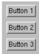
Figure 4–1 An example of a vertical frame from FXVerticalFrame .
