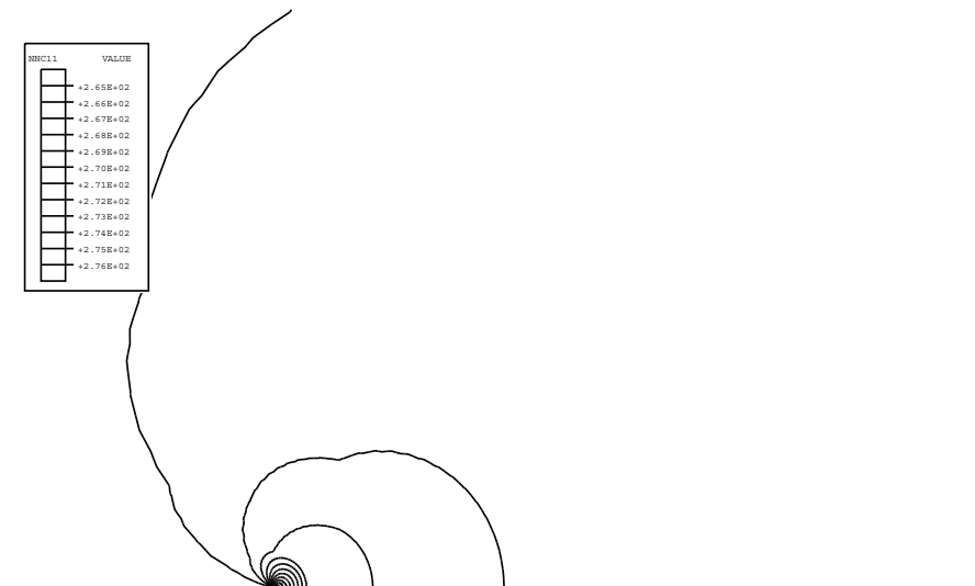
Figure 8.1.2-4 Contours of normalized hydrogen concentration at the crack tip.
