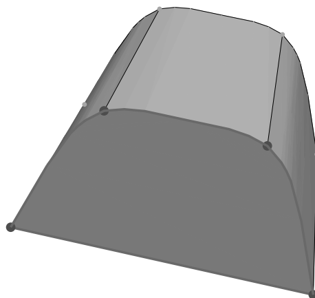
Figure 17–100 Faces with corner radii may require editing for use as connecting sides.
