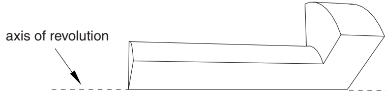
Figure 17–76 Abaqus/CAE cannot mesh a region with hexahedral elements if one or more edges lie along the axis of revolution.
